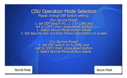
Once the download is complete – it should automatically proceed to this screen. To enable the CDU Security function, you'll want to choose 'Secure Mode' from the menu, however follow the instructions and set the switches before doing so.
