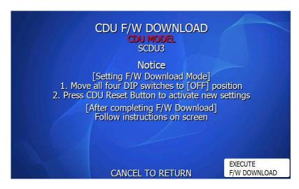
Follow the steps on the screen and move all 4 switches to the 'Down' position. Press the Reset button once you've done that.
