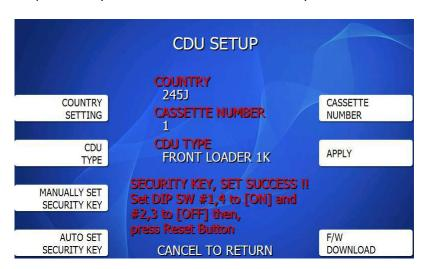
Per the instructions above – now change the switches to #1, #4 up and #2, #3 down and press the reset button.
